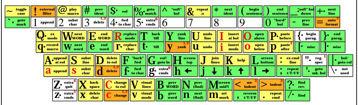
motion moves the cursor, or defines the range for an operator
